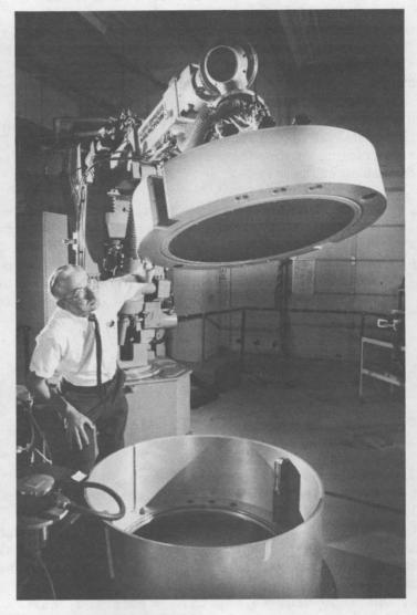
EXTENDED FAMILY of "smart" robots is helping automate a variety of DOE operations. In Sandia's robot lab, researchers are developing a system that inspects lids on transport casks for high-level radioactive waste. Ben Petterson (1416) is seen checking the underside of a full-scale model of such a cask lid at Sandia's inspection station. (See "Automated Handling Techniques Reduce Waste, Hazards" on page five.) (Photo by Randy Montoya, 3162)
